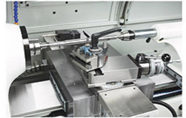
Lathe center in tailstock single tool on quick change tool holder on compound tool slide.
