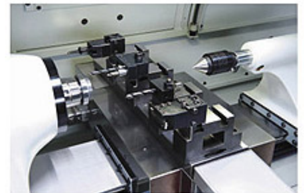
Multiple "single" gang tool plates each holding a single tool holder.
