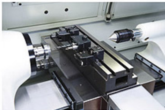
One full length gang tool plate with T-slots to accommodate different kinds of tool holders.
