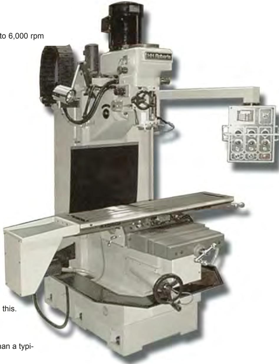
In this photograph the TW-32-Q is shown with the standard chip pan. Larger chip pans and side splash guards are available as shown on the TW-50-RH on the next page. Also on current models the spindle speed and direction controls are placed on the head, not in the pendant as shown in the pictures.
