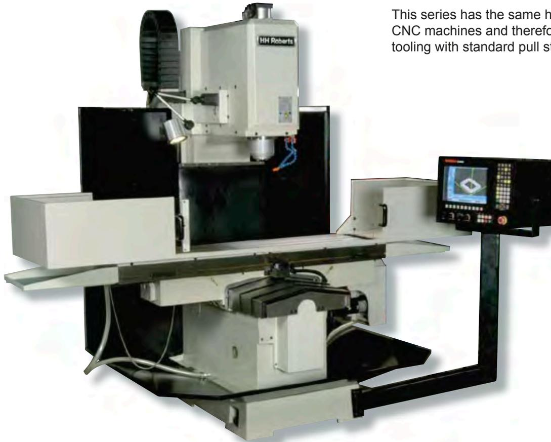
This series has the same heads and spindles as our CNC machines and therefore uses CAT-V40 or BT-40 tooling with standard pull studs.
