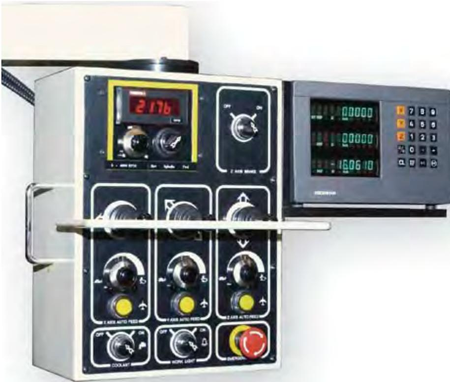
The pendant has the spindle speed display at the top left.
