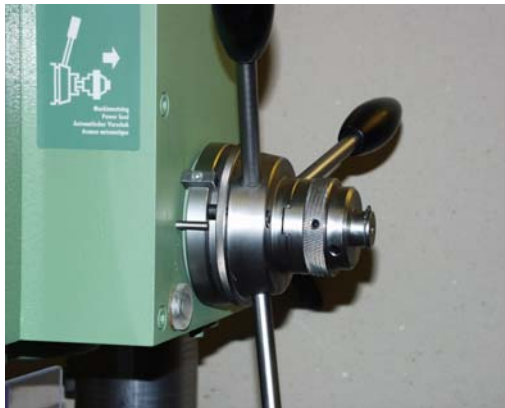
Picture 2. Inserted coupling
