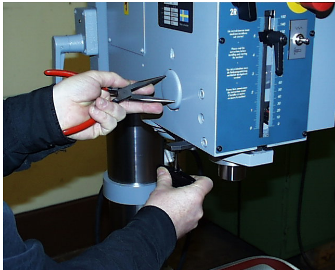
Picture 5: Removing the spring case
