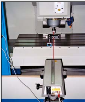
Laser Linear inspection (ISO 10791-4)
