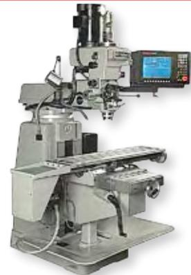
2 and 3 axis knee mills with tilting heads or rigid heads up to 7 1/2 Hp and 40" x 20"
