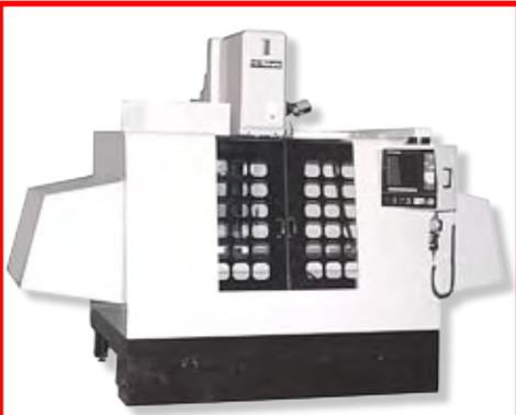
Vertical machining centers, open and enclosed 31" x 20" to 60" x 32"
