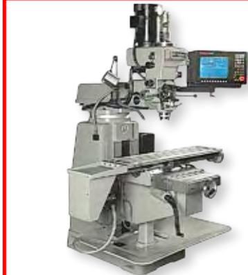
2 and 3 axis knee mills with tilting heads or rigid heads up to 7 1/2 Hp and 40" x 20"
