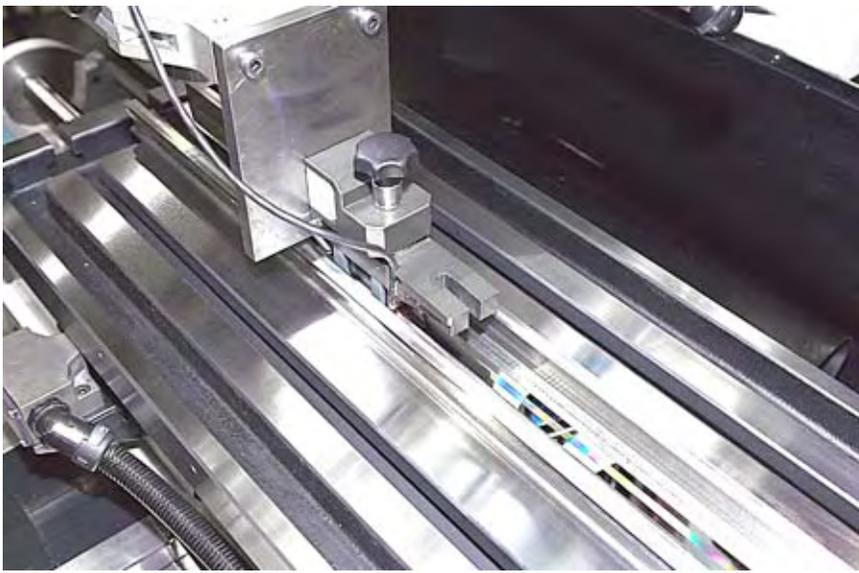
The Heidenhain VLM scale during inspection for positioning and repeatability.
